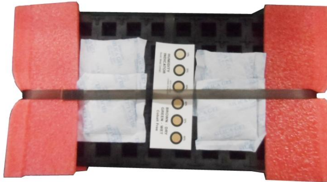
Figure 2-4 Arrangement of the modules (after the vacuum bag is removed)
