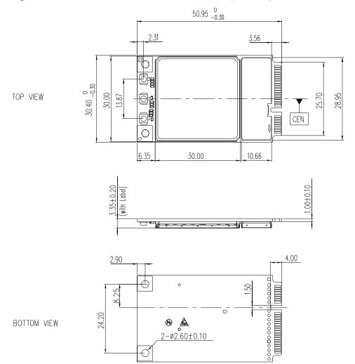
Figure 6-1 Dimensions of the ME909u-521 module (unit: mm)
