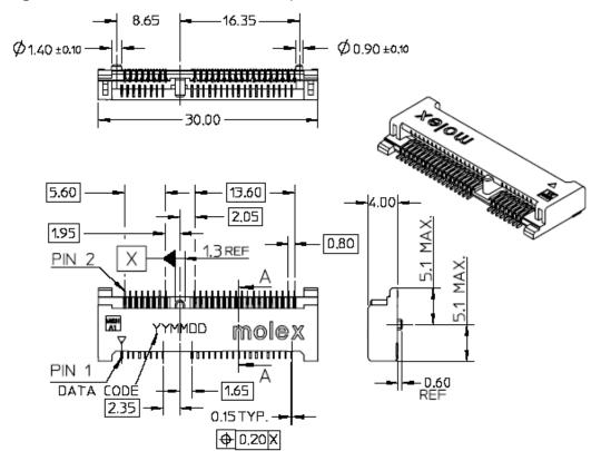
Figure 6-2 Dimensions of the Mini PCI Express connector
