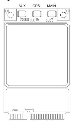
The antenna connectors must be used with coaxial cables with characteristic impedance of 50  $\Omega$ .
