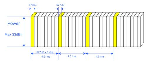
For general packet radio service (GPRS), the uplink transmission uses two or more successive time slots, as illustrated in Figure 2-2.
