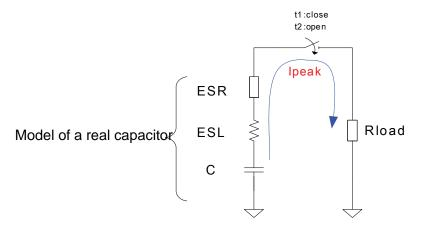
Assume that the original voltage on the ideal capacitor is Vo and the peak current is  $\mathbf{I}_{peak}$ . When the power supply switch is turned off, the capacitor starts to release electric charge. Before the switch is turned on, the voltage on the load  $(\mathbf{V}_{load})$  can be calculated using the following formula:
