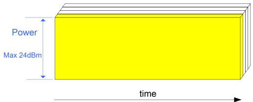
For Huawei modules operating on the WCDMA and FDD-LTE networks, when the transmitted power reaches the maximum transmitted power, the required maximum current from the power supply is approximately 1100 mA. Therefore, power supplies with an average output of at least 1.5 A are required.
