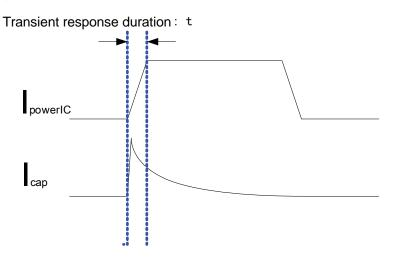
Figure 3-5 illustrates that the peak current is provided by the compensation current  $(I_{cap})$  from the capacitors when the power supply IC is in the transient response duration. After the transient response duration, the capacitors can stop the output current. Note that Figure 3-5 does not consider the case that the power supply IC will charge the capacitors after the transient response duration.
