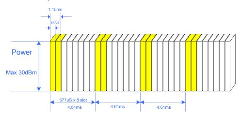
Figure 2-2 GPRS uplink transmission
