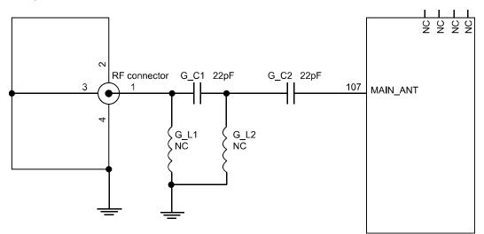
**Figure 3-19** RF signal layout design about MAIN\_ANT for reference:(the same for AUX & GPS)
