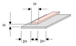
Figure 3-21 Complete structure of the stripline
