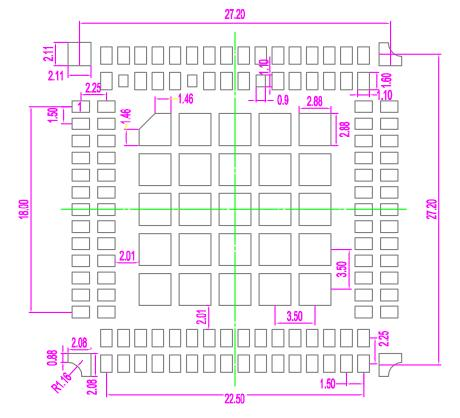
Figure 6-5 Footprint design of customer's PCB (unit: mm)
