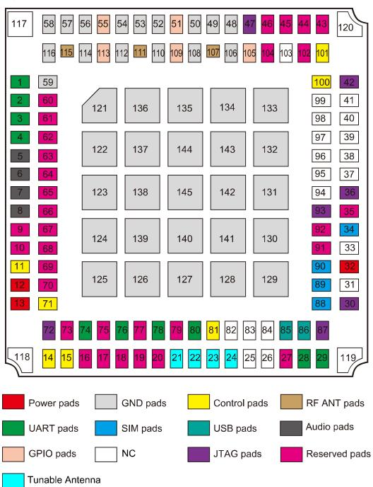
Figure 3-1 Sequence of LGA interface (Top view)
