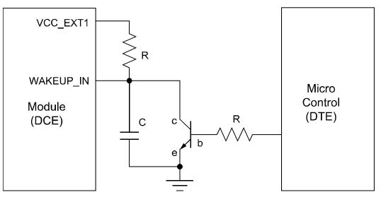
The pull up resistor should not be greater than 22 k $\Omega$ .
