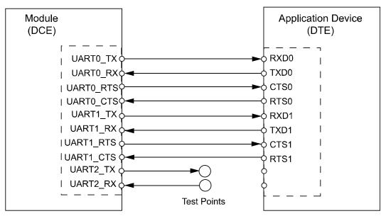
The RS-232 chip can be used to connect the ME909u-521 module with UART. In this connection, the Complementary Metal Oxide Semiconductor(CMOS) logic level and the Electronic Industries Association (EIA) level are converted mutually. For example,
