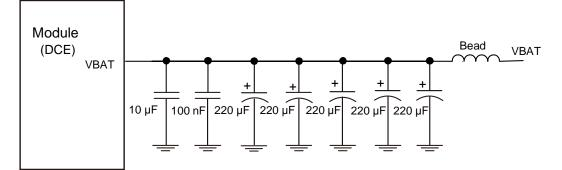
When the system power restarts, a discharge circuit is recommended to make sure the power voltage drops below 1.8 V and stays for 100 ms at least. This is very important. If POWER\_ON\_OFF is asserted when the VBAT is between 1.8 V to 3.2 V, the module may enter an unexpected status.
