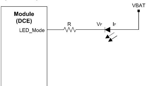
Figure 3-12 Driving circuit
