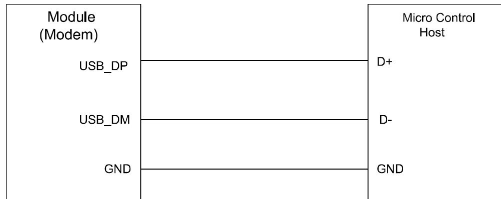
Figure 3-8 Recommended circuit of USB interface
