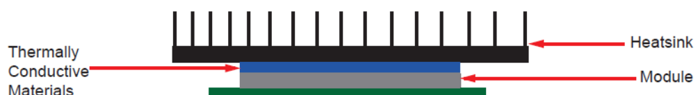
Figure 6-4 Adding a heatsink to the module for optimal heat dissipation
