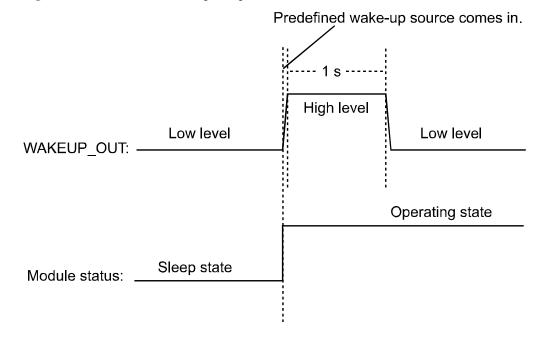
Figure 16-1 WAKEUP\_OUT output sequence
