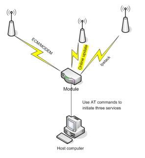
When multiple host computers run AT commands to use the same APN to initiate dial-up connections for different services, the connections share a bearer.
