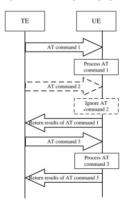
Figure 1-2 AT command processing sequence diagram
