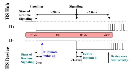
Figure 16-7 Successful procedure of remote wake-up
