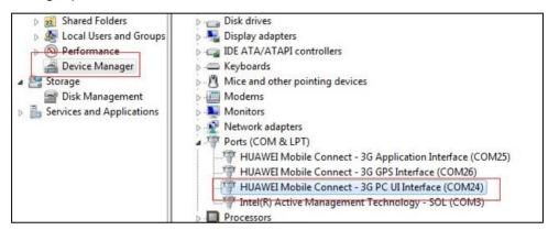
Step 2 Run a serial port application such as HyperTerminal to open the GPS port.
