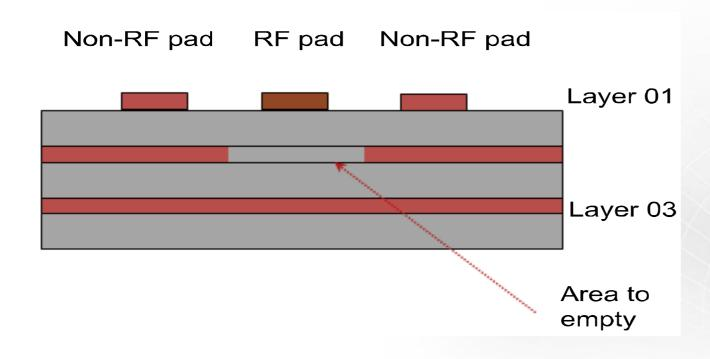
[RF Rule2] The recommended distance between the RF pad and copper sheet in the same layer is 15 mils.
