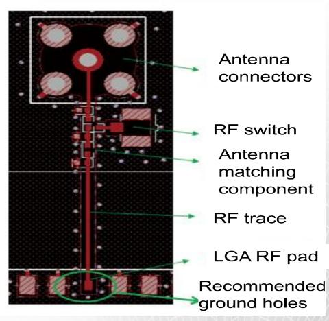
[RF Recommendation5] For SMA connectors, the distance between the RF pad and surrounding sheet is 100 mils. And the ground holes are well-distributed around.
