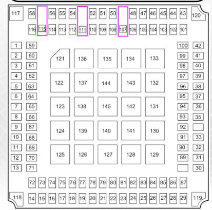
[RF Rule1] For boards that have more than two layers, empty part of the adjacent layer below the RF pad. Emptying method: Empty the copper sheet of the adjacent lower layer. The area to empty is 30 mils larger than the RF pad.
